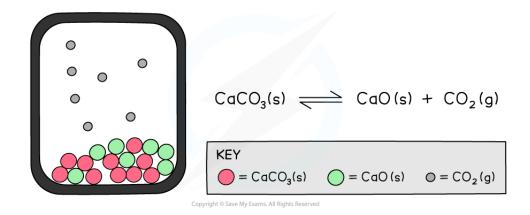
The diagram shows a closed system in which no carbon dioxide gas can escape and the calcium carbonate is in equilibrium with the calcium oxide and carbon dioxide
